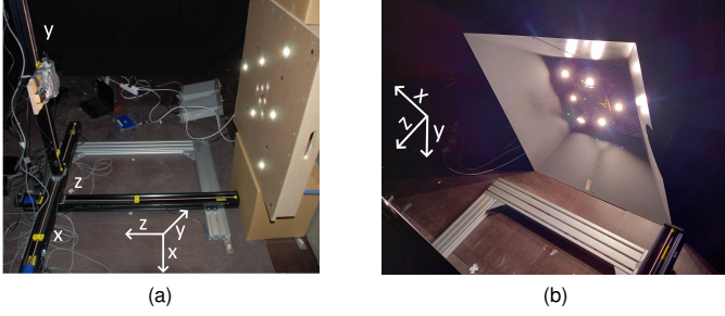
Fig. 1. Visualisation of the (a) flat surface and (b) drone funnel landing zone with the measurement setup (i.e. the Velmex slider system) present.
