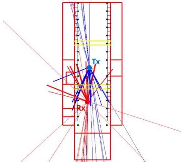
■ Example: time delay dispersion at repair shop
